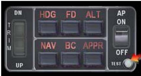
Preflight test determines, before takeoff, that the FDS is operating normally. With avionics power ON, AP Servos (AP) OFF, both engines started, Autopilot/FD circuit breakers IN, and gyros to speed, depress the TEST button. A normal test will be observed when each mode indicator illuminates in sequence, followed by an audible annunciation.
