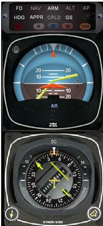
The approach mode provides visual roll and pitch commands on the FCI V-bar to capture and track precision ILS/LOC and glideslope beams.
