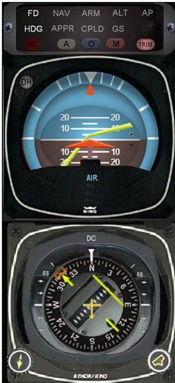
Select the desired heading by turning the OBS knob on the HSI. The heading bug will turn to the selected heading.
