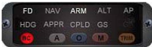
Whenever an LOC or ILS frequency is selected, the BC mode may be activated by depressing the BV button on the CMU. The ARM light will illuminate.
