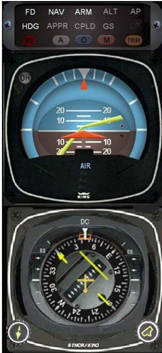
The NAV mode provides bank commands and deviation guidance on the HSI to intercept and track a VOR.
