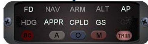
Whenever a condition exists while the FDS is in VNAV (ALT) mode where the vertical trim cannot be validated the TRIM light will illuminate on the annunciator.
