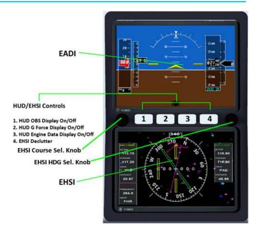
The Primary Flight Display (PFD) provides all the information displayed on a traditional airspeed indicator, attitude indicator, altimeter, vertical speed indicator, horizontal situation indicator, and turn coordinator in a modern, easy-to-scan format featuring a large horizon that's easy to see. The PFD also displays communication and navigational radio information, flight plan data, an inset moving map, outside air temperature, transponder status, and time of day.
