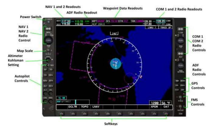
The Multi Function Display (MFD) combines engine information with a full-featured GPS and moving map display. You can obtain a zoom in view of the MFD by clicking the moving map area.
