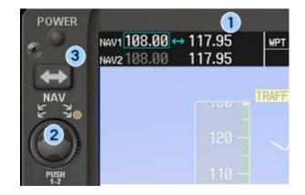
The NAV radios are on the upper left corner of the PFD. The COM radios are in the upper right corner. The radio frequency window (1) displays active and standby frequencies for dual receivers for both NAV and COM, as well as the identifier of a valid, identified navigation aid. The active frequency of each radio is on the right and the standby frequency is on the left. The cyan-colored tuning box indicates which standby frequency will be set using the NAV knob.
