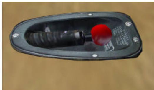
When electric failure has occurred or the electric system has been turned off, the Manual Gear Pump Lever will now look as follows:
