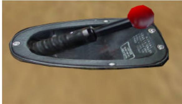
When the Manual Gear Pump Lever is in the up position because of a generalized electric failure and your intention is to lower the landing gears, it is important that you pull/lower the main landing gear lever to the extend landing gear position. This will allow for the correct positioning of the gear valves (if you do not take this step you will not be able to manually lower the landing gears).
